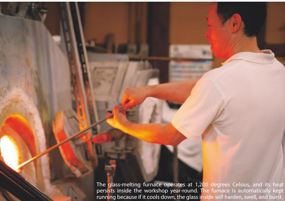
The glass-melting furnace operates at 1,200 degrees Celsius, and its heat persists inside the workshop year-round. The furnace is automatically kept running because if it cools down, the glass inside will harden, swell, and burst.
